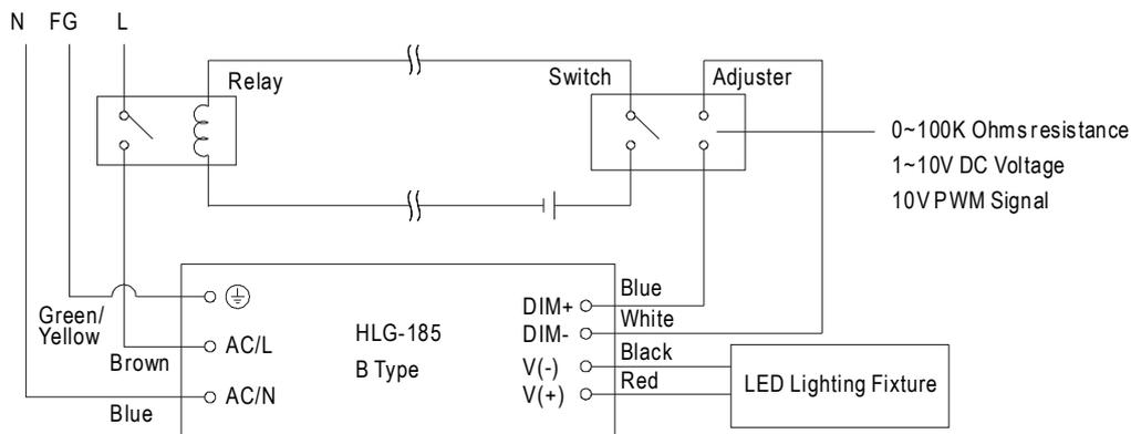
Using a switch and relay can turn ON/OFF the lighting fixture.
